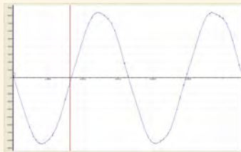
Output VSD Voltage Waveform with Inversine ( V_{THD} < 3\% Typical)
