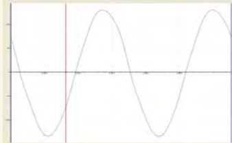
Output VSD Current Waveform with Inversine I_{THD} < 8\% Typical
