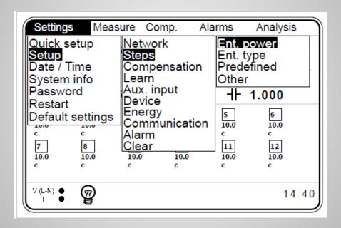
Note: The PFW03-M24 has 2 power inputs. In the "Ent. Power 1" submenu, the operator enters the powers into the 1st, 2nd... and 12th steps, and in the second Submenu "Power 2", into the 13th, 14th... and 24th steps.
