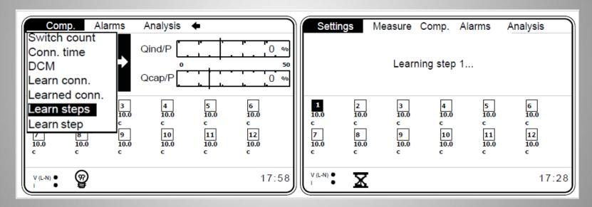
NOTE: No load (current and amplitude) must present changes in the system to ensure that the step powers are learned correctly. Otherwise, the PFW03 may learn the step powers incorrectly.
