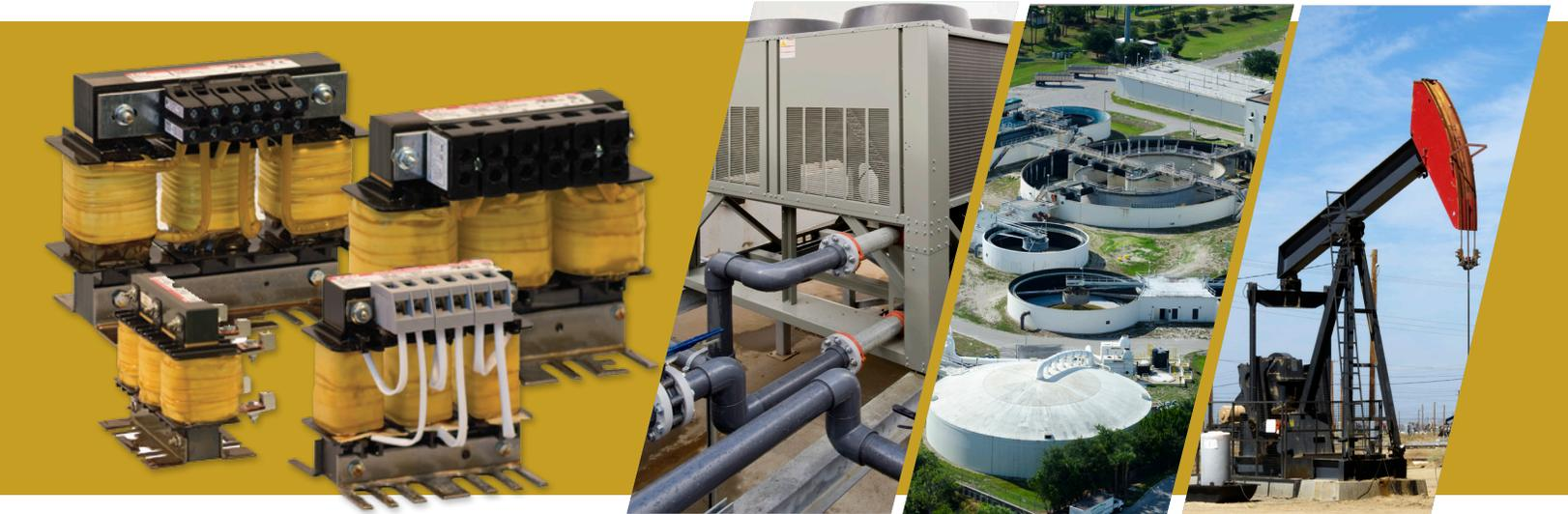
KDR line reactors are electrical components that help to protect 6-pulse rectifiers and power conversion devices such as variable frequency drives (VFDs). When used in conjunction with a VFD, a KDR line reactor can help reduce harmonics and protect the drive from harmful voltage spikes. KDR line reactors are recommended on the input of each VFD in multiple drive applications.
