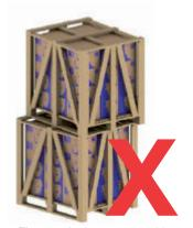
Figure 5.2 - Incorrect stacking
