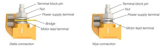
Figure 6.13 - Connetion for W21 and W22 motors with terminal block
