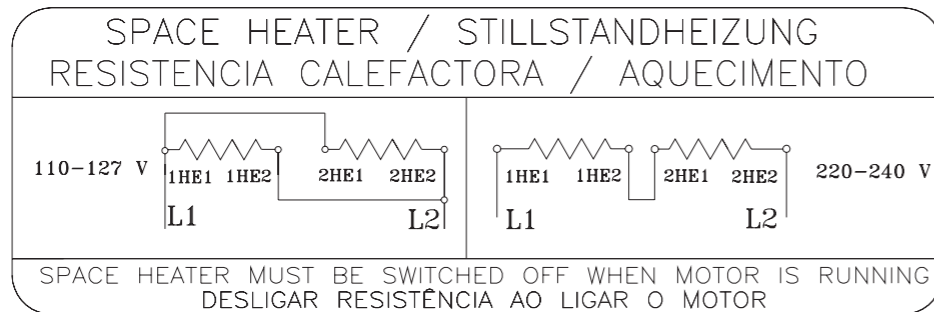
Figura 6.18 - Dual voltage space heater connection.
