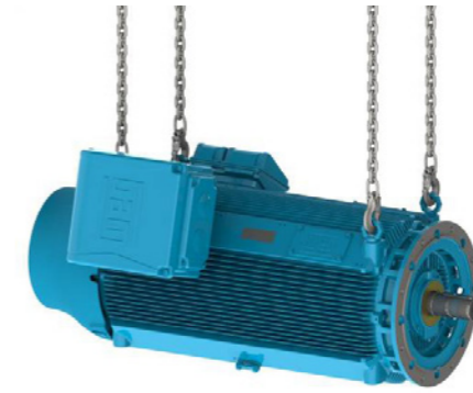
Figure 4.13 – Lifting of HGF and W50 motors with two hoists
