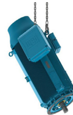
Figure 4.15 - Lifting HGF and W50 motors by the eyebolts at the non-drive end
