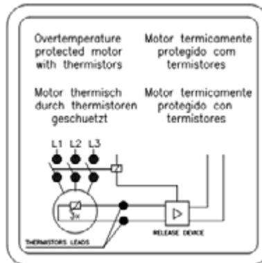
Figure 6.17 - Thermistor connection
