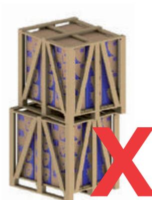
*Figure 5.2 - Incorrect stacking*
