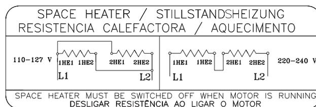
Figure 6.19 - Dual voltage space heater connection
