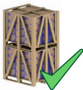
*Figure 5.1 - Correct stacking*
