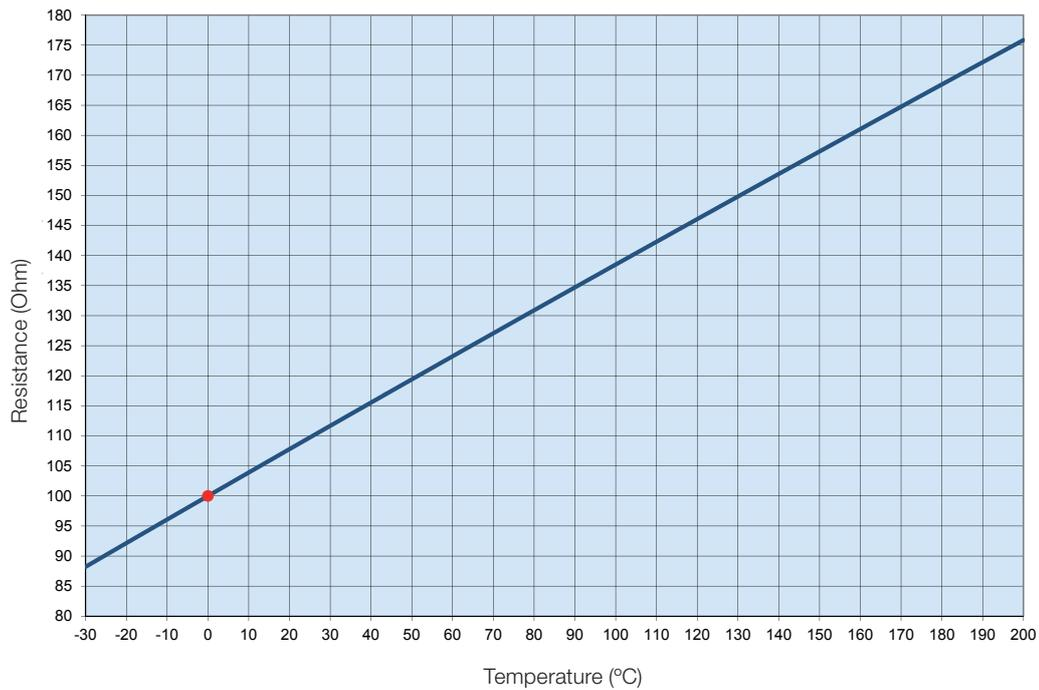
Figure 6.18 - Ohmic resistance of the Pt-100 x temperature
