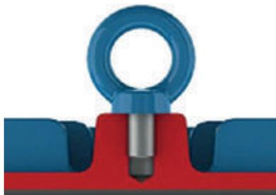
Figure 4.1 - Correct tightening of the eyebolt
