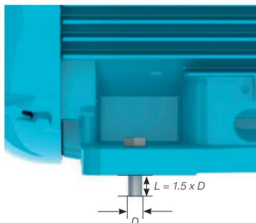
Figure 6.6 - Mounting system of a foot mounted motor
