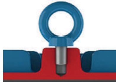
Figure 4.2 - Incorrect tightening of the eyebolt
