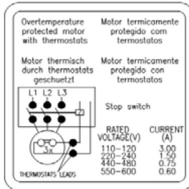
Figure 6.16 - Connection of the bimetal thermal protectors (thermostats)
