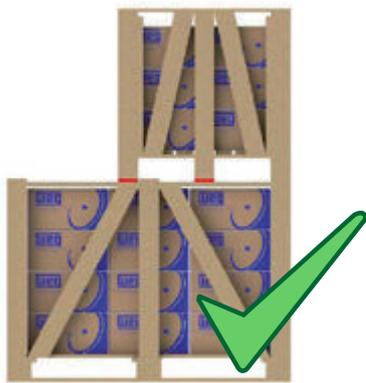
Figure 5.3 - Correct stacking
