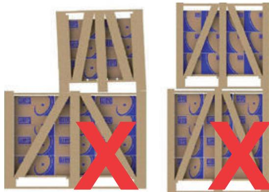
Figure 5.4 - Incorrect stacking
